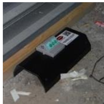
Detector mounted on an upturned length of plastic guttering
