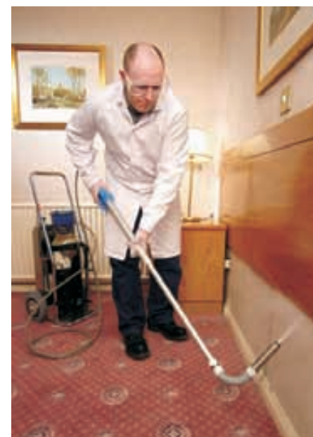
The Cryonite method uses the extreme cooling properties of liquid CO 2 to freeze the bedbugs to death
