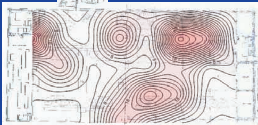
The contour map highlights hot-spots of activity. Overlaying it onto a site plan pinpoints areas, or items of equipment, where infestation is most concentrated
