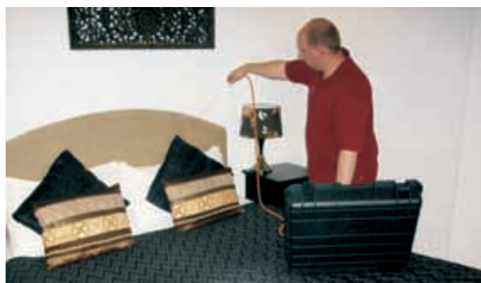
Air samples are taken using the specialist portable sampling machine
