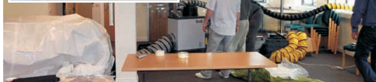
Hands-on activity on the BPCA course. Main picture: Introducing the heat to the sheeted stack. Inset: Sheeting up and inserting temperature probes into the stack
