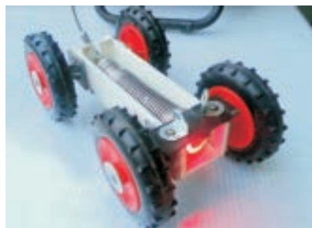
Meet 'drain rover', Justin's homemade answer to transporting 'sewer cam'
