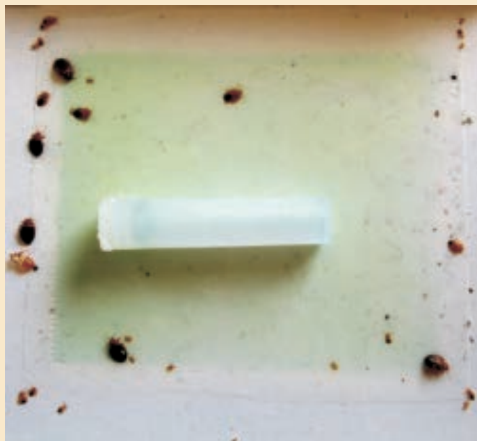
An opened Suterra monitor, clearly showing the lure plus bed bugs and nymphs on the adhesive
