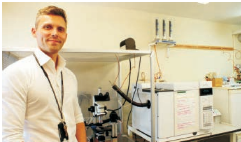
Coupled gas-chromatography electroantennography, where electrodes are attached to an insect's antenna to identify novel attractants and repellents is another piece of specialist kit available
