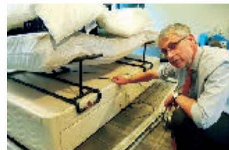
Good air circulation is vital so as to ensure all items achieve maximum temperature. Three heat probes check for this
