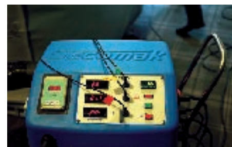
The control panel displays the temperature of each of the three probes
