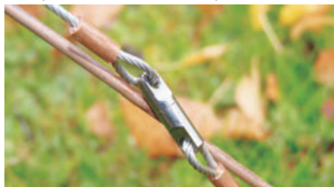
The two swivels allow the fox to twist and spin without kinking the wire
