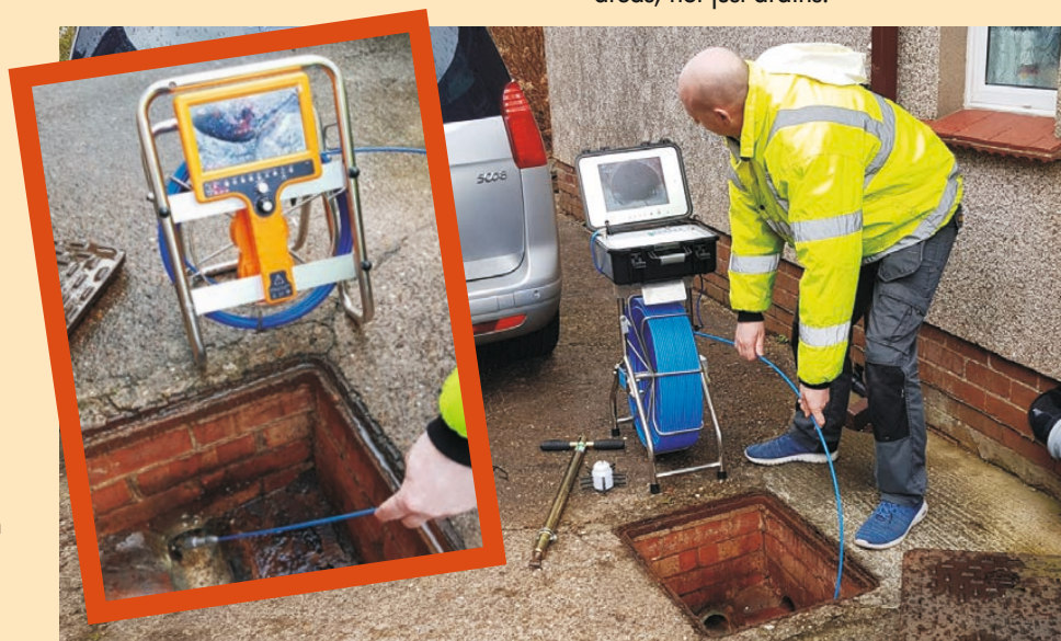
The portable IPL 20 produces high quality images and carries ample lighting to illuminate larger pipes but the small diameter rod is more at home in smaller pipes
