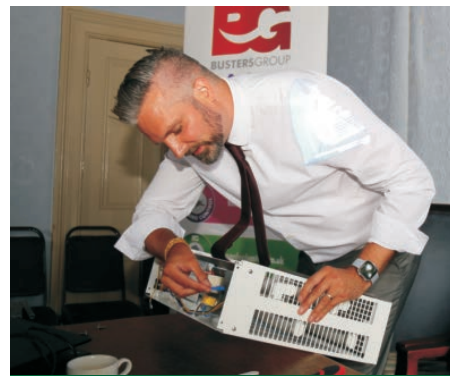
David Haskins showing the inner workings of the Insect-a-Clear machine, pointing out the ballasts and transformer
