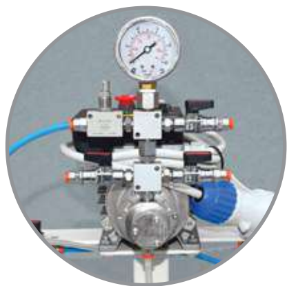
Detail of the supply and pressure valves
