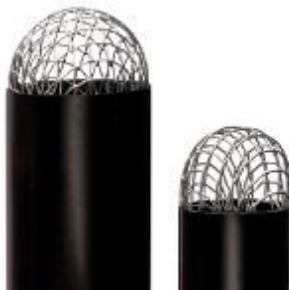
Wire balloons prevent rat emergence from sewer vent pipes. Plastic balloons are less effective as rats can chew through them
